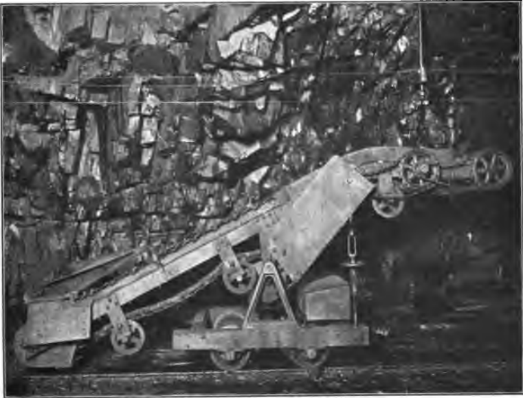
PORTABLE LOADER AT THE NORTH LAKE MINE OF THE CLEVELAND-CLIFFS IRON Co., ISHPEMING, MICH.
